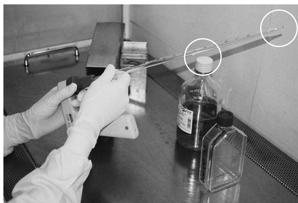
Fig. 5.9. Inserting a Pipette in a Pipette Controller. Pipette being inserted correctly with grip high on the pipette (above the graduations) and the pipette pointing away from the user. Circled areas mark potential risks, namely inadvertently touching the bottle or the back of the cabinet.
