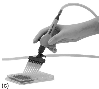
Fig. 4.9. Aspiration of Medium. (a) Pipette connected via tube to a peristaltic pump being used to remove medium from a flask. (b) Peristaltic pump on the suction line from the hood leading to a waste receiver. (c) Withdrawal of fluid from multiwell plate (same adapter can be used with regular pipettes and flasks), and (d) vacuum pump receiver (courtesy of Integra.)
