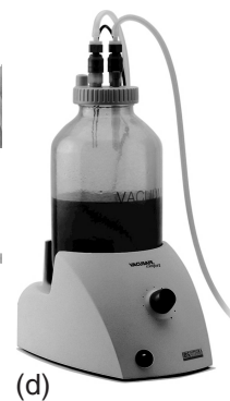
Fig. 4.9. Aspiration of Medium. (a) Pipette connected via tube to a peristaltic pump being used to remove medium from a flask. (b) Peristaltic pump on the suction line from the hood leading to a waste receiver. (c) Withdrawal of fluid from multiwell plate (same adapter can be used with regular pipettes and flasks), and (d) vacuum pump receiver (courtesy of Integra.)
