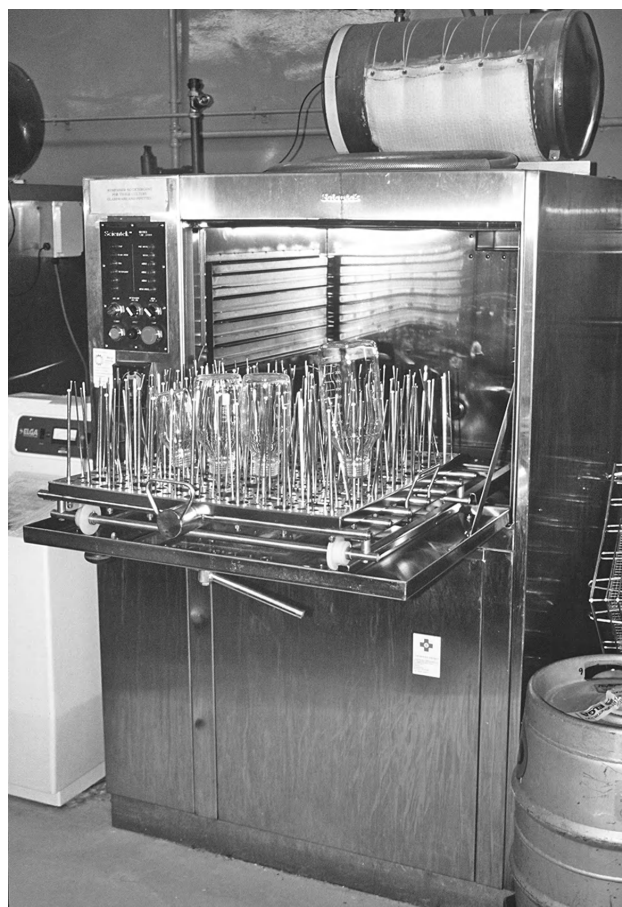
Fig. 4.14. Glassware Washing Machine. Glassware is placed on individual jets, which ensures thorough washing and rinsing (Betterbuilt). (Courtesy of Beatson Institute.)
