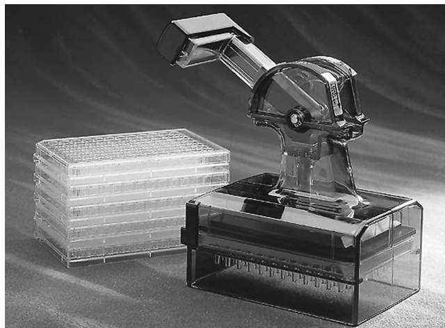
Fig. 4.8. Transfer Device. Transtar (Corning) for seeding, transferring medium, replica plating, and other similar manipulations with microtiter plates, enabling simultaneous handling of all 96 wells. (Reproduced by permission of Corning Life Sciences.)
