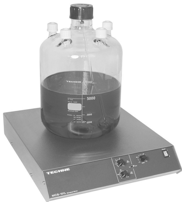
Fig. 26.1. Large Stirrer Flask. Large stirrer flask (5 L) on a magnetic stirrer. Note the offset pendulum that makes an excursion in the annular depression in the base of the flask. The side arms are for sampling or perfusion with CO 2 in air, which would be required with this volume of medium (see Fig. 26.2) (Techne, courtesy of Sterilin.)
